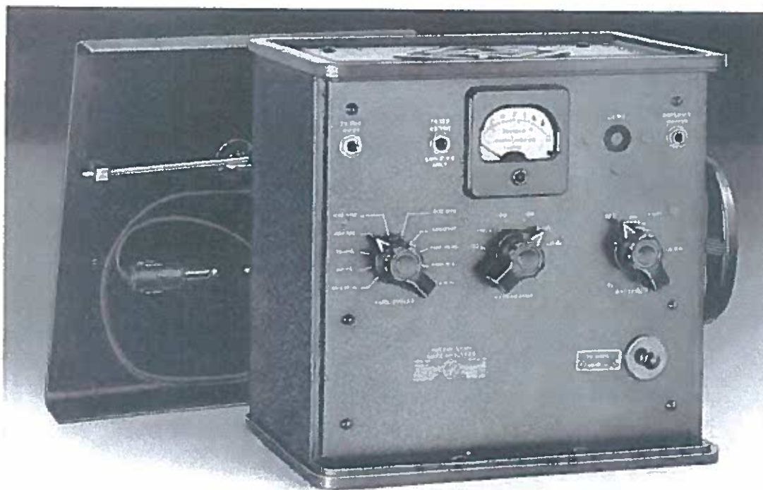
Figure 1. View of the Type 1550-A Octave-Band Noise Analyzer with cover removed to show panel.
